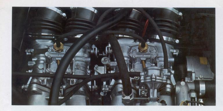
Engine: 4-cylinder, 4-stroke in-line engine. Hemispherical combustion chamber, overhead camshaft, inclined valves in V-arrangement, crankshaft mounted in five bearings, water cooled, force-feed oil lubrication by geared pump and micronic main flow filter
